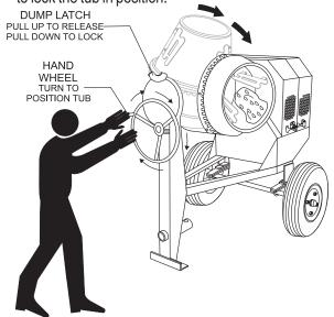
Figure 19. Mixing Drum Positioning
